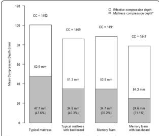
**Fig. 2** Mean chest compression depth in four study conditions. Legend: \*percentage represents proportion of mattress compression depth over total compression depth. CC number of compression
