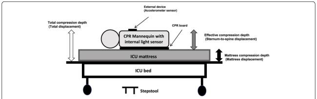
**Fig. 1** Description of study setting. Legend external device—measuring total displacement (effective compression depth+mattress compression depth); internal light sensor—measuring sternum-to-spine displacement of the mannequin (effective compression depth); mattress compression depth = total compression depth—effective compression depth
