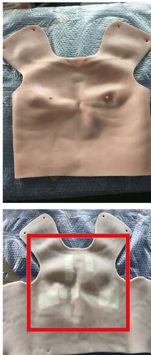
Fig. 1 Prototype wearable auscultation vest (top, visible surface; bottom, underside) with embedded panel speakers at the anatomically-standardized auscultation positions (red box)
